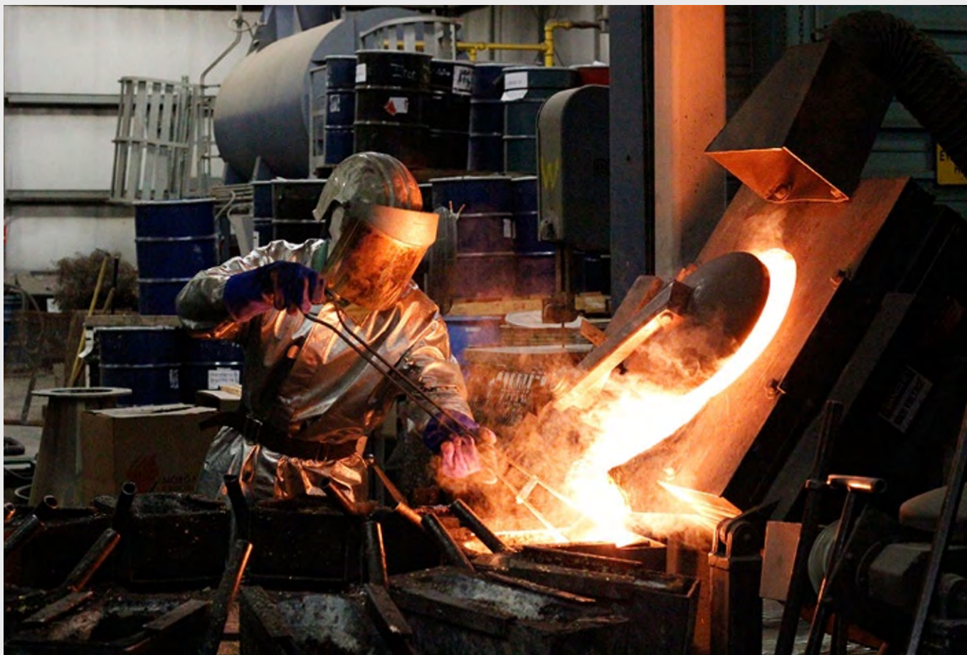
Fig 3. Pyrometallurgical processing of PGM-containing materials
